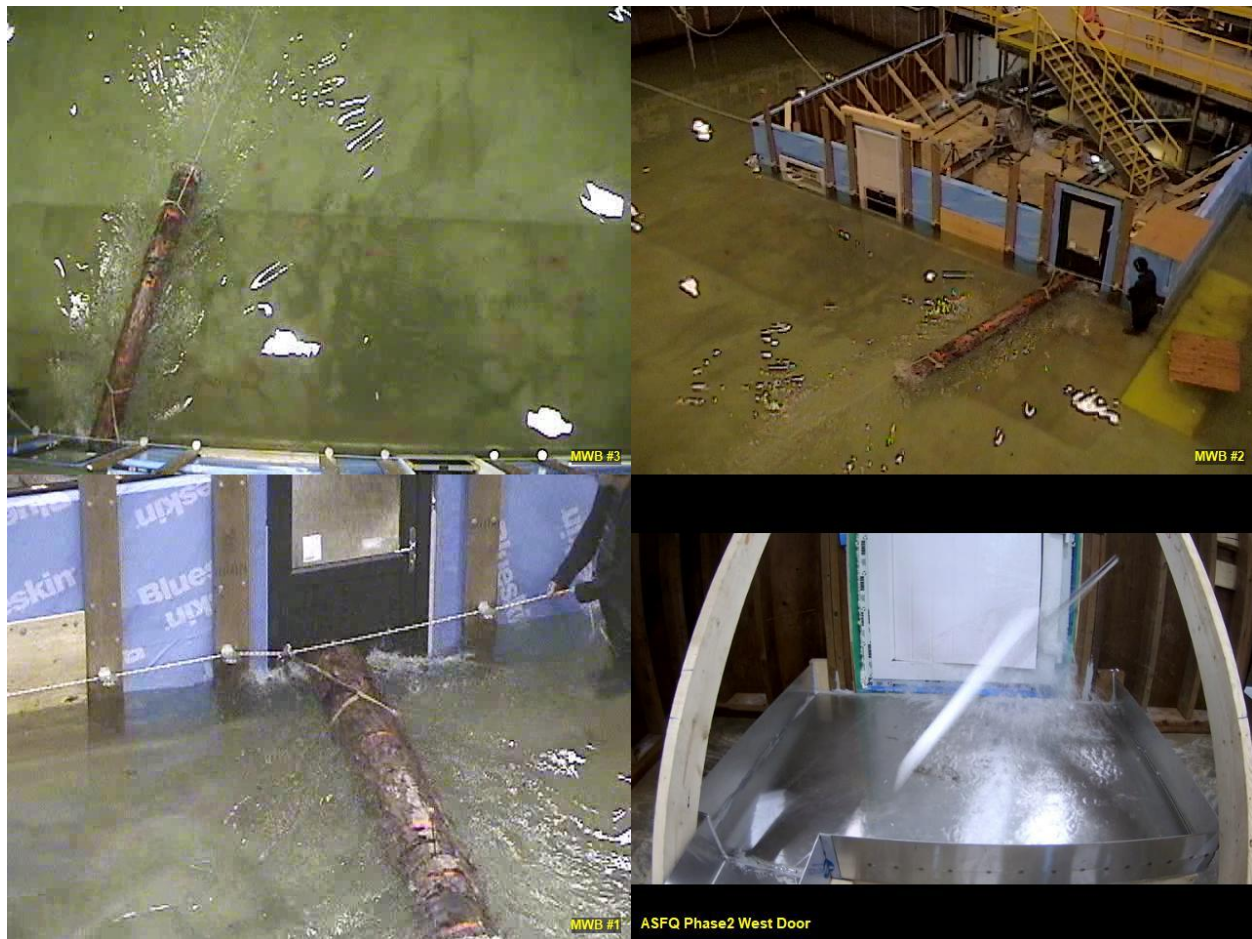
Figure 48. Failure of the StormMeister door under debris impact.
