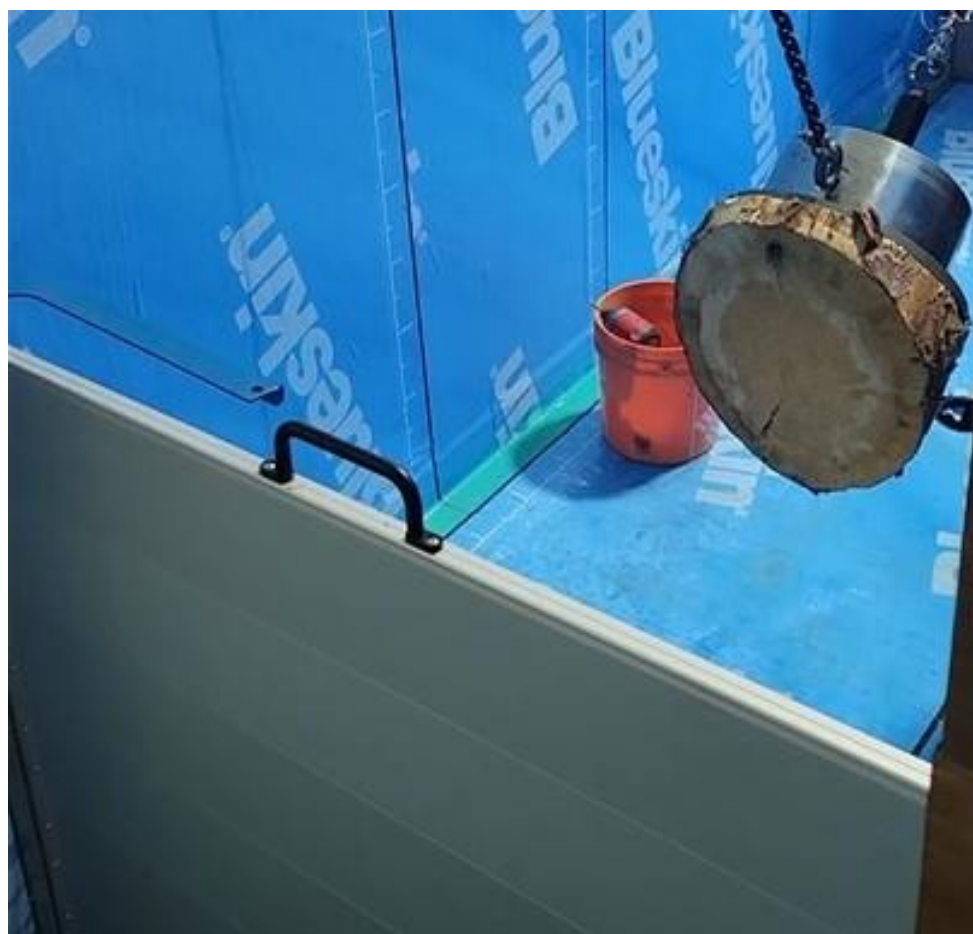
Figure 31. Debris impact testing in Phase 2 in the Ice Tank.
