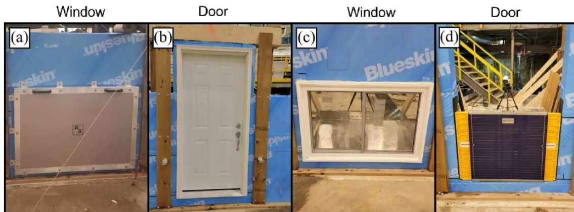
Figure 21. Opening barriers deployed in the MWB in Phase 2 – second set of tests: (a) RS Stepanek; (b) Standard Door; (c) Sliding Window; and (d) DamEasy.
