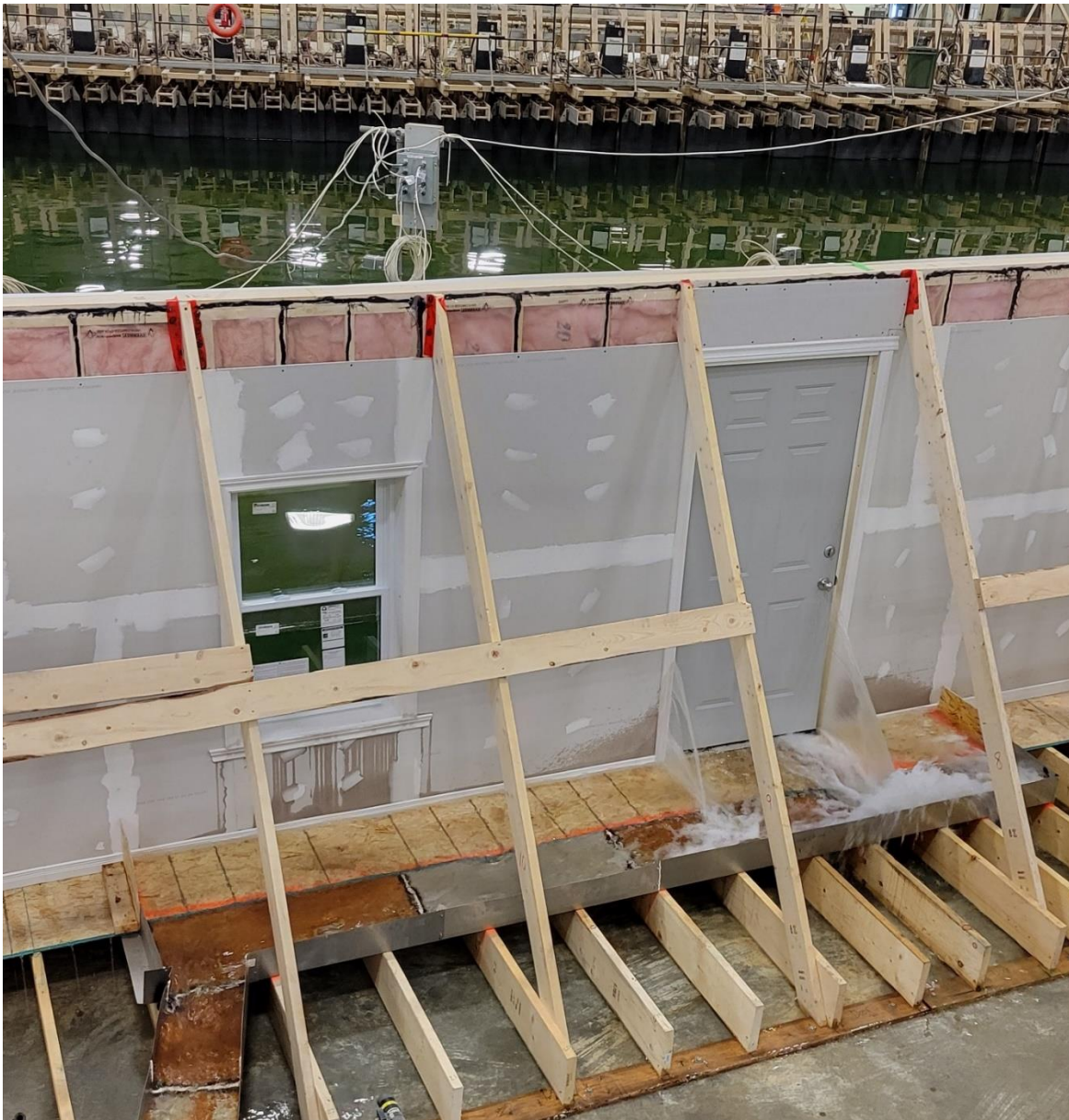
Figure 33. Leakage through the door observed in Phase 1 at maximum water depth.
