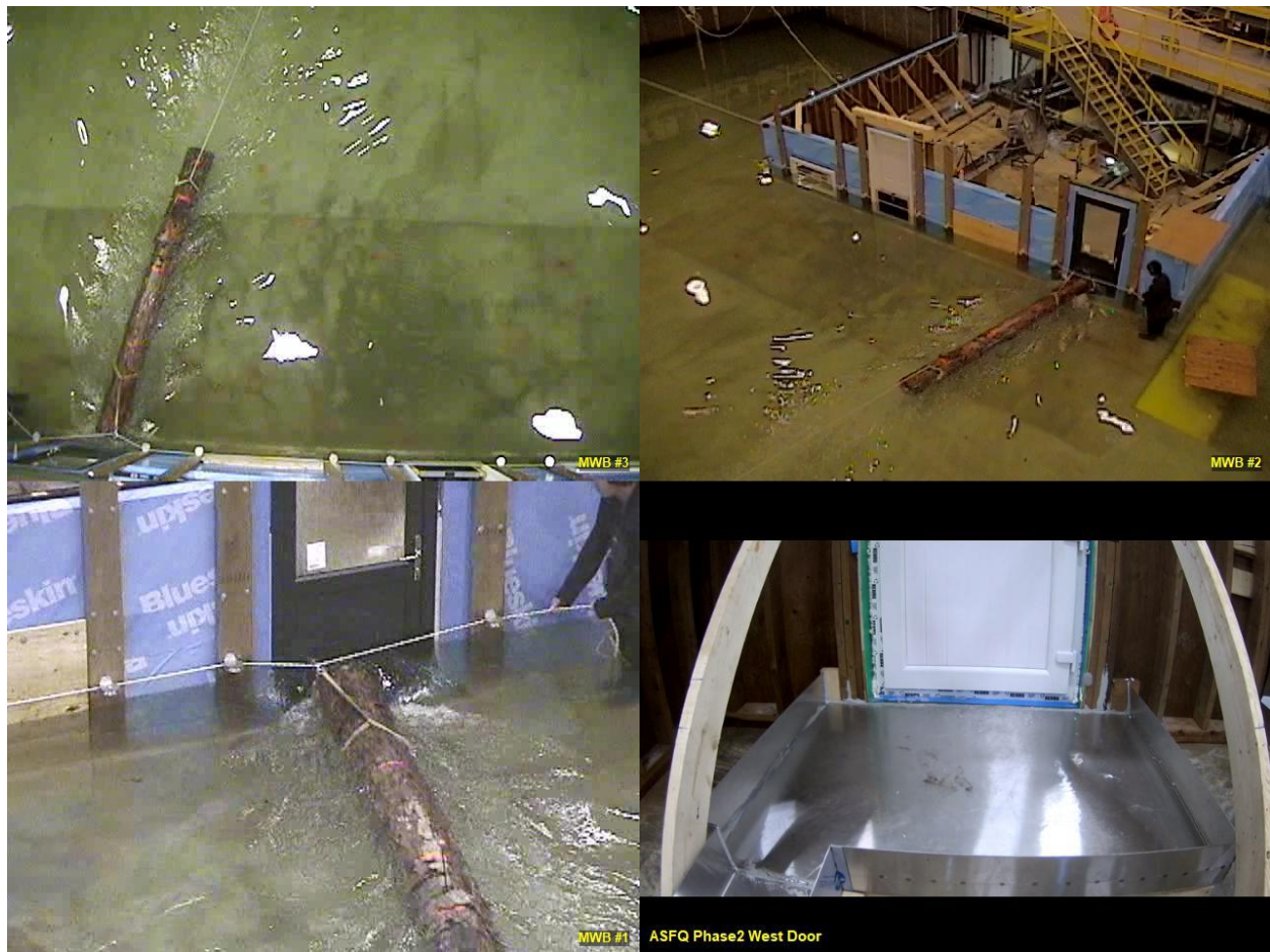
Figure 47. Debris impacting the StormMeister door just prior to failure.
