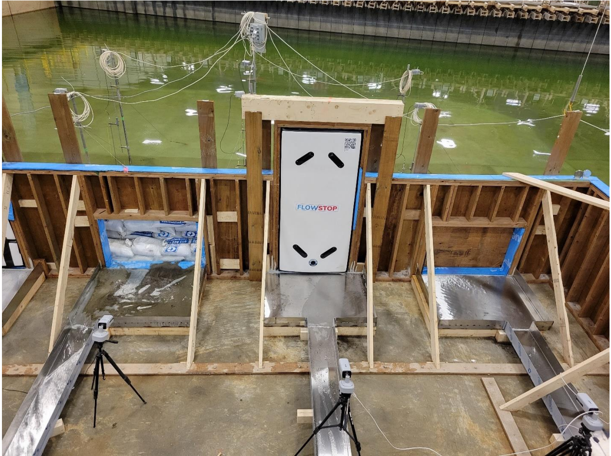
Figure 28. An image of performance testing of flood protection measures, from left to right sandbags, FlowStop full-sized cushion and plywood.
