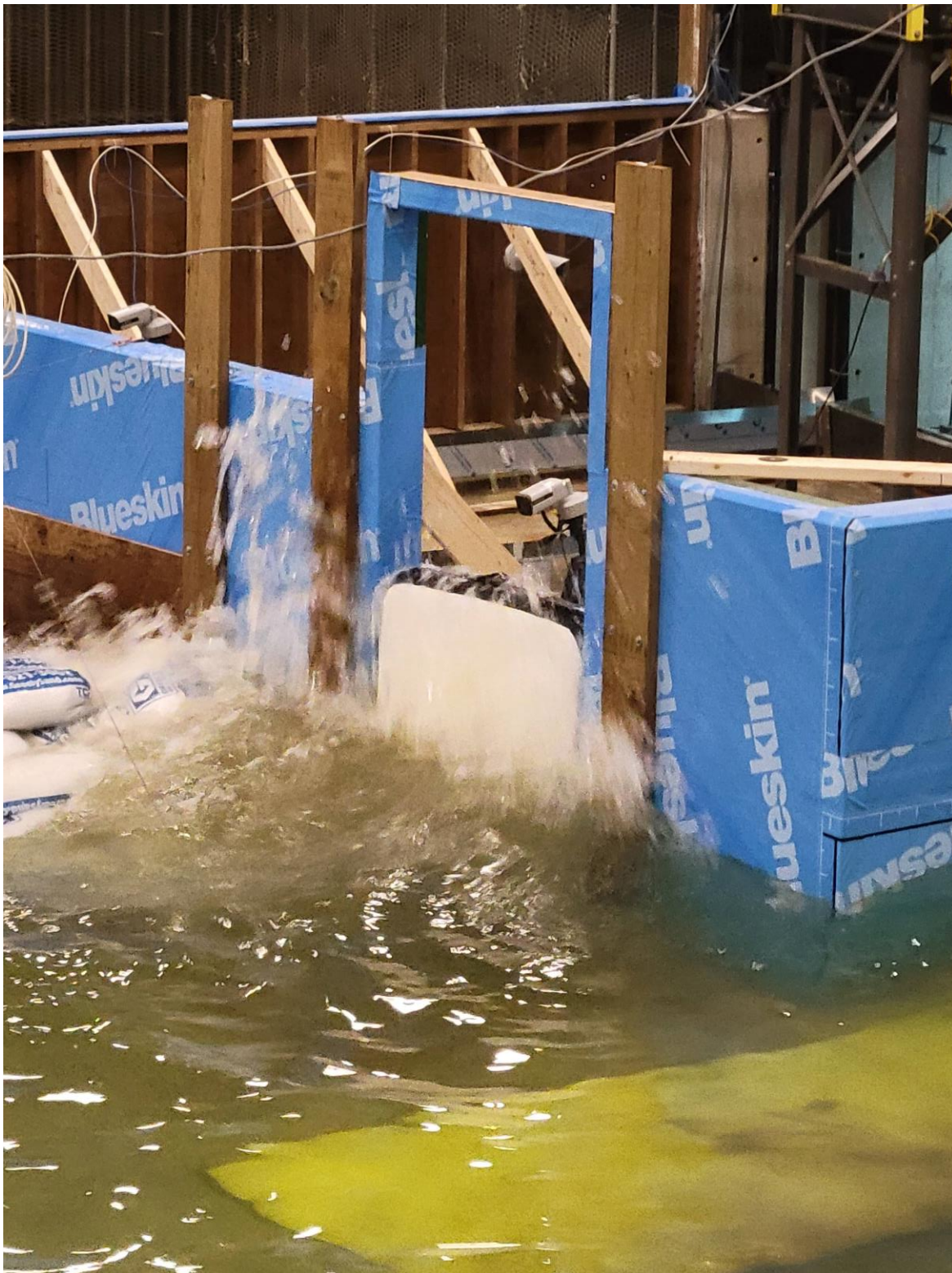
Figure 25. Image from Phase 2: TSE – west door, waves overtopping the FlowStop regular cushion.
